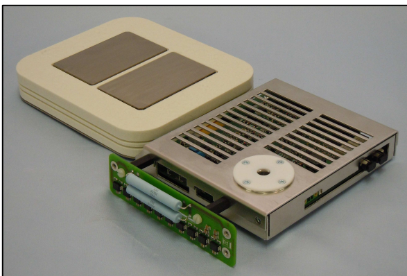
Figure 5. 5SNA 1250K450300 with gate unit and clamp resistors
