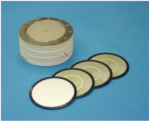
Fig. 6: ABB p/n 5SPB 36Z1350 prototype with Diode and switching wafers
