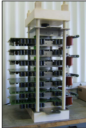
Fig. 6. Reverse Conducting Switch Assembly complete P/N 5SVG 073508E01
