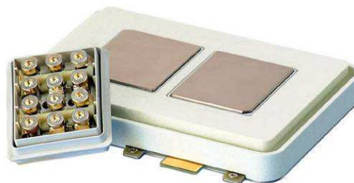
Fig. 11. Sub Module Emitter Side (1200A pulse rating) Complete Module Collector Side
